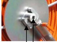
HOSE REEL SHAFT METAL FITTING HOOK
